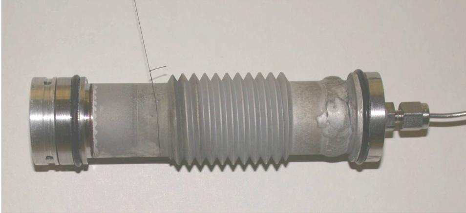
FIGURE 2. Assembled [F-18]fluorine gas target.
